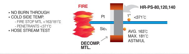
**FIRE SEAL** SURFACE BURNING CHARACTERICS TEST (ASTM E84)
